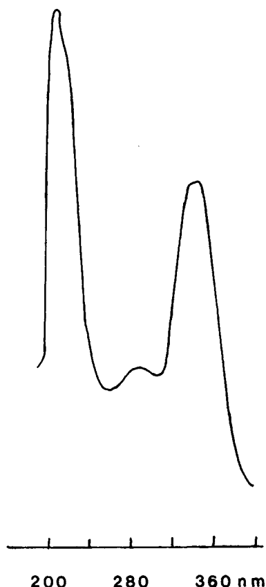
Figure 1 UV spectrum of the cooligomer formed by the reaction of Jeffamine -2000 and trimethylhexamethylene diamine with p -benzoquinone. The 344 nm peak represents substituted quinones and the 291 nm one probably the presence of hydroquinone.
